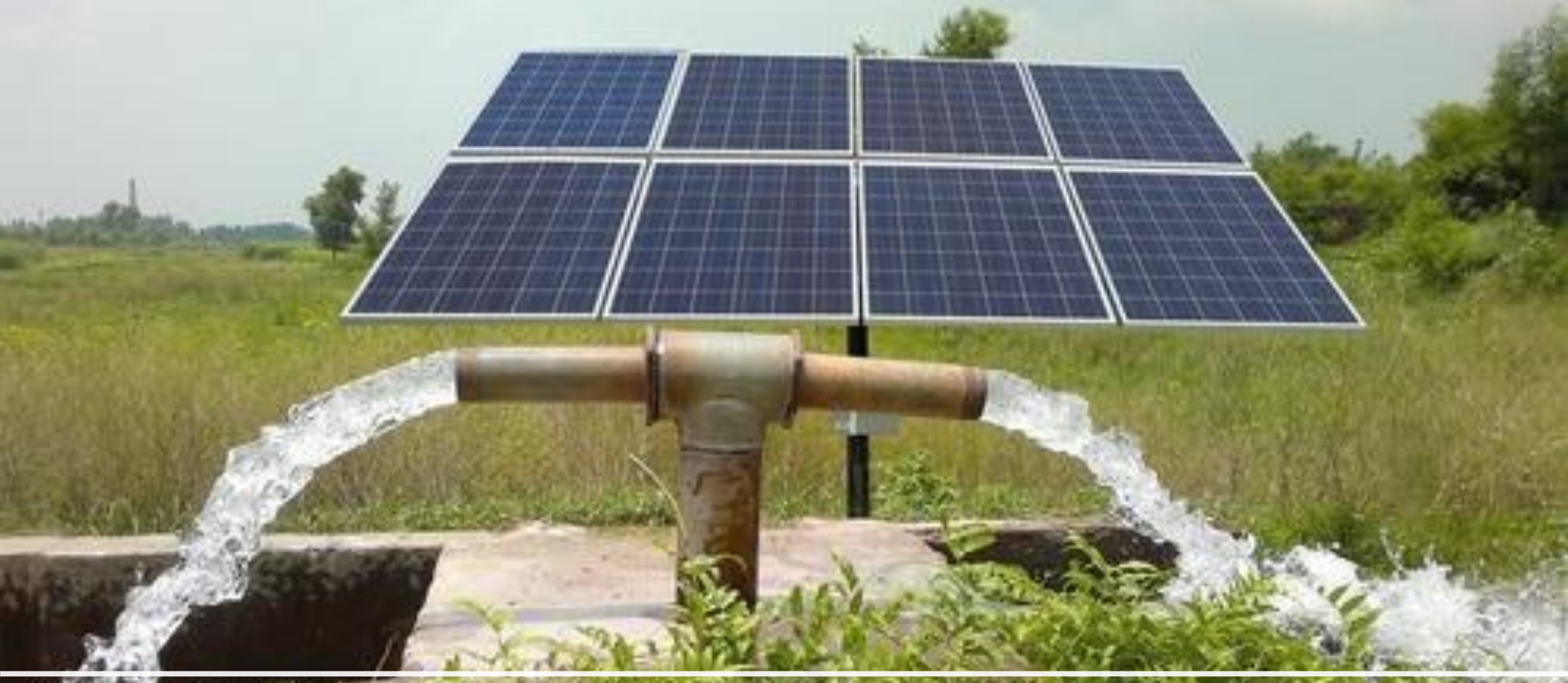
SOLAR WATER PUMP
